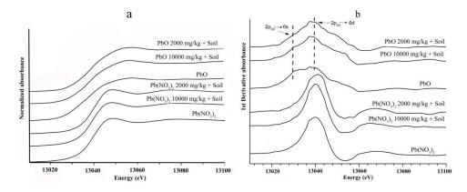
Figure 2. The experimental Pb  $L_{III}$ -edge XANES spectra (a) and their first derivatives (b) for the reference compounds (PbO and Pb(NO<sub>3</sub>)<sub>2</sub>) and the Pb-treated soil samples
