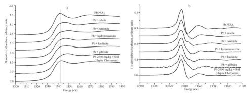
Figure 4. (a) Experimental Pb  $L_{III}$ -edge XANES spectra and (b) 1-st-derivative X-ray absorption spectra for soil, layered silicate phases, and Pb(NO<sub>3</sub>)<sub>2</sub> standard
